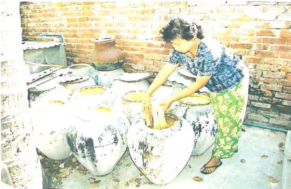
**Photo.2. Putting the small bamboo bundles into the pots with Lime**
