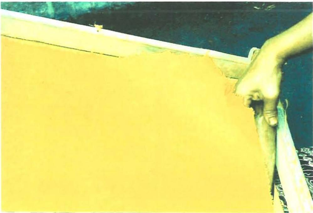
Photo.23. Peel off the paper from the frame
