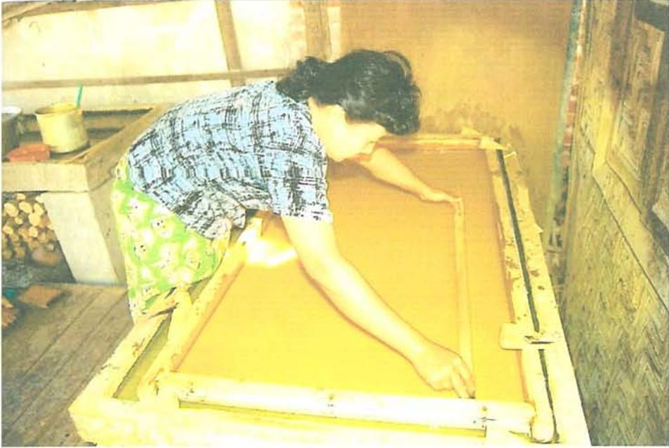
**Photo.9. Spreading the cloth sheet with bamboo pulp with a round stick**
