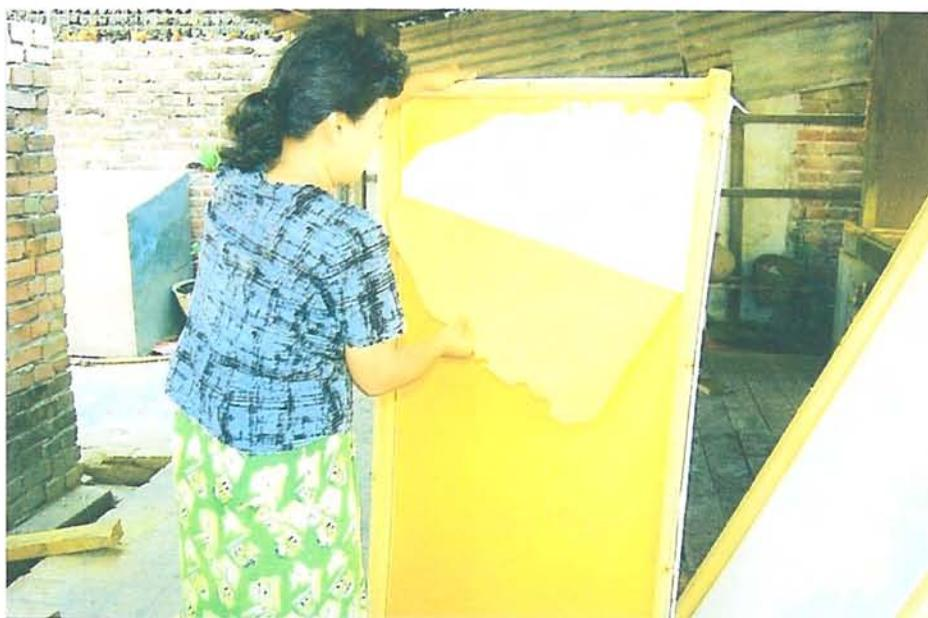
**Photo.12. Peel off the cloth from the frame**
