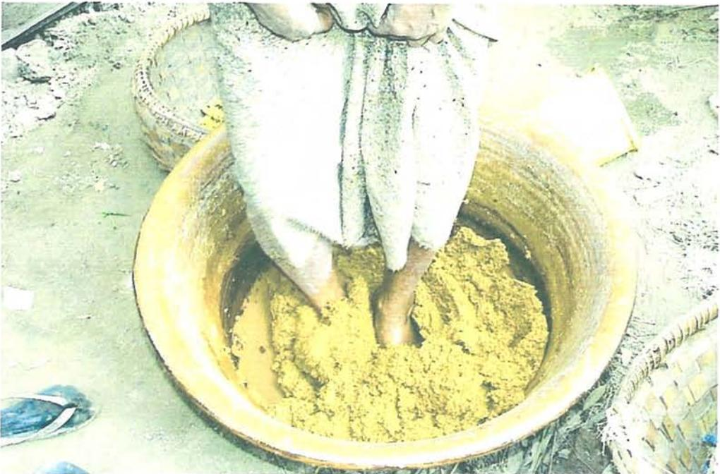
**Photo.19. Pressing the pounded pulp into a pot**
