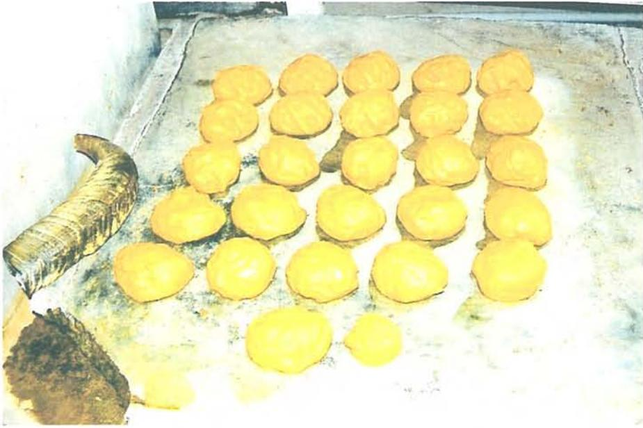
**Photo.5. Balls of bamboo pulp**
