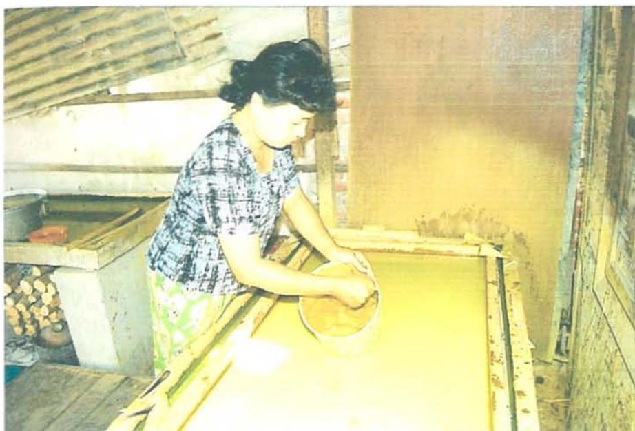
**Photo.7. Balls of bamboo pulp mixed with a bit of water and stirred with a *Dalet***
