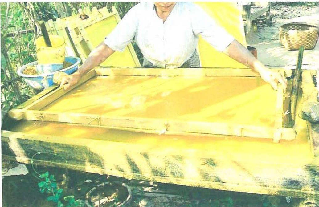
**Photo.21. Pouring the liquid of pulp onto a cloth**
