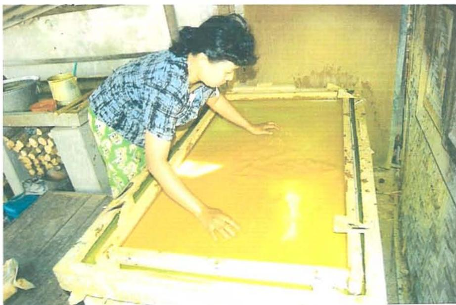
**Photo.8. Spreading bamboo pulp mixture on a teak wood frame**
