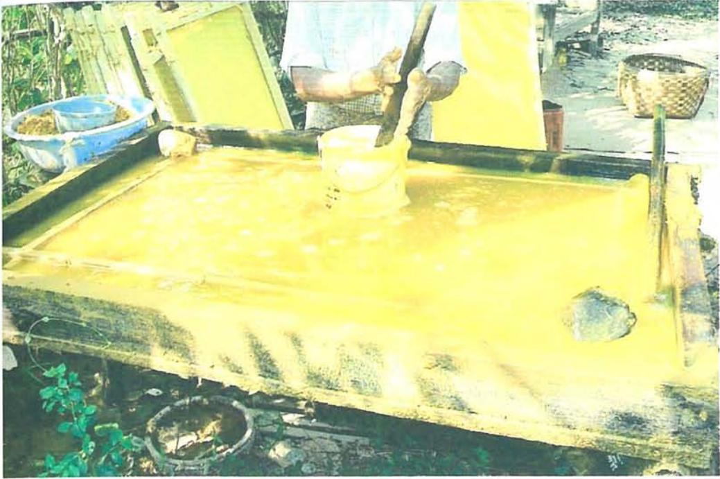
**Photo.20. Mixing the 10-ticals of pulp with water**
